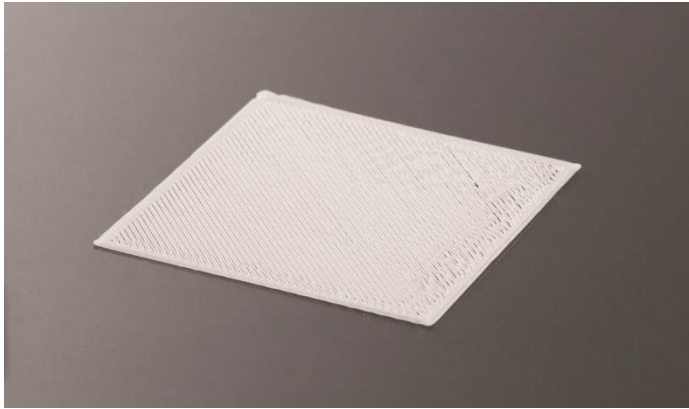
Fig. 44 Example of a too low position of the heatbed
